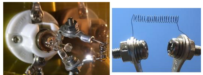
Figure 6 Schematic of thermionic emission experiment (top), and electron gun (bottom)
