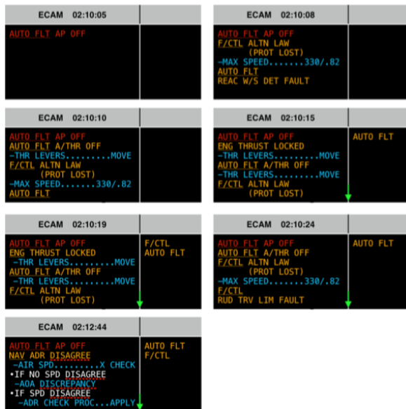
Figure 5 ECAM screen display at time of incident [11]
