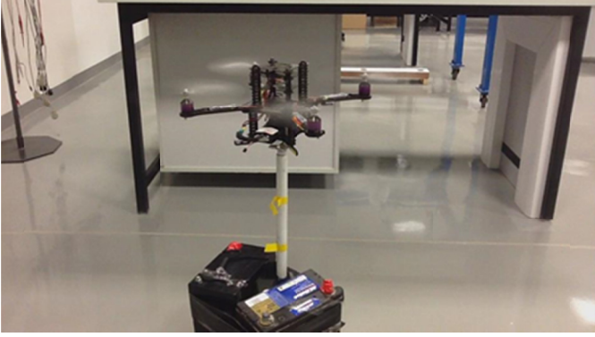
Figure 7 – Testbed for testing attitude stabilization of the quad-rotor
